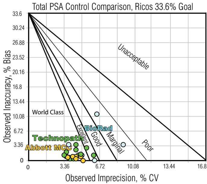
Figure A29. Six Sigma Method Performance comparison of Bio-Rad, MCC (Bio-Rad) and Technopath controls for Total PSA.
