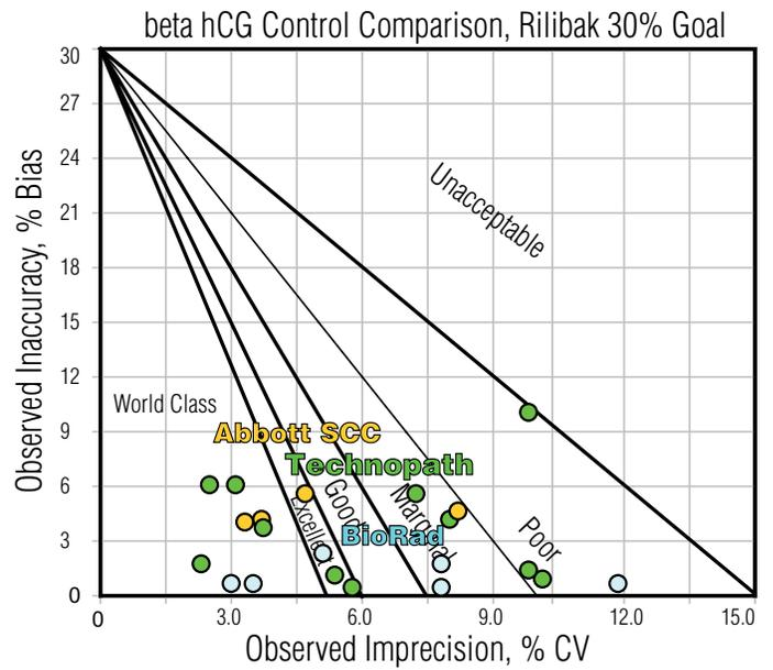
Figure A30. Six Sigma Method Performance comparison of Bio-Rad, Abbott SCC and Technopath controls for beta hCG.
