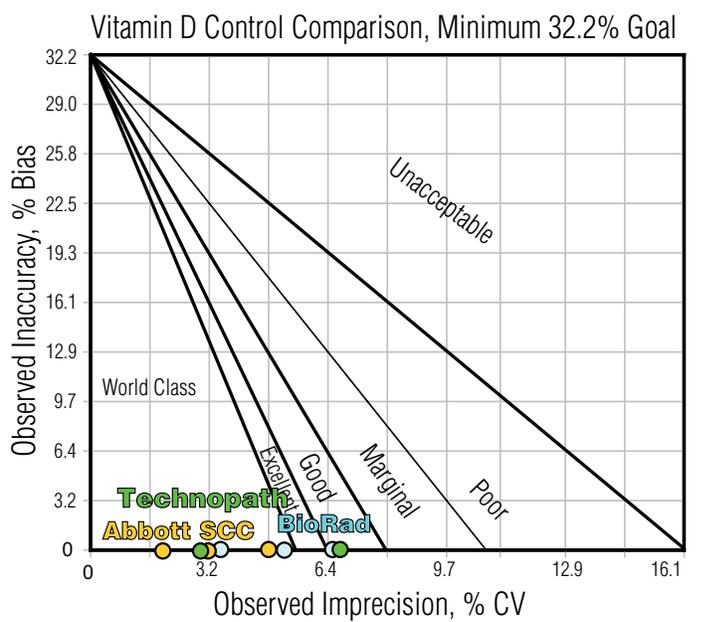
Figure A32. Six Sigma Method Performance comparison of Bio-Rad, Abbott SCC and Technopath controls for Vitamin D.
