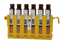
Up to six quality controls vials can be loaded on a single rack and up to four racks can be loaded on the instrument.
