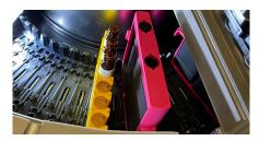
Quality controls can be stored onboard the system, in a temperature controlled reagent carousel, and automatically run at user-defined intervals.
